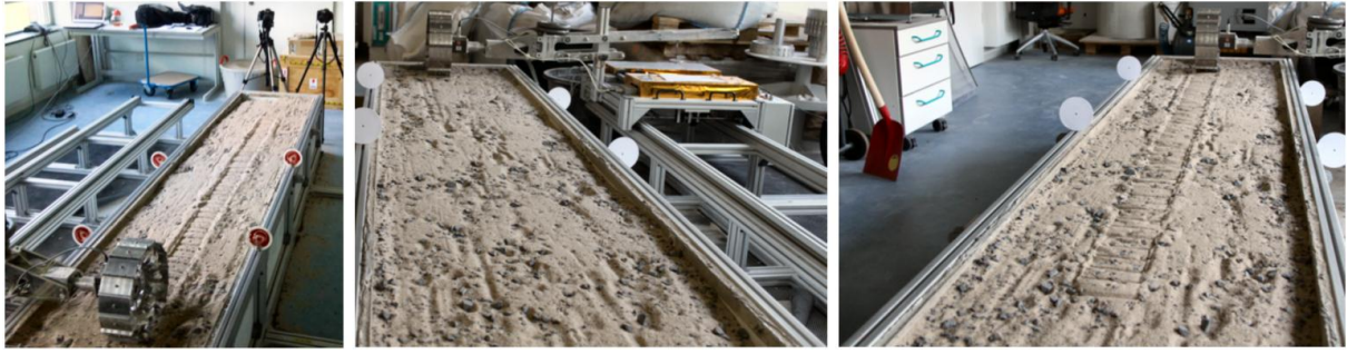
Figure 23: Left: Experimental setup with stereo cameras visible in the background. Middle, right: Stereo images of track region (left image without track, right image with track)
