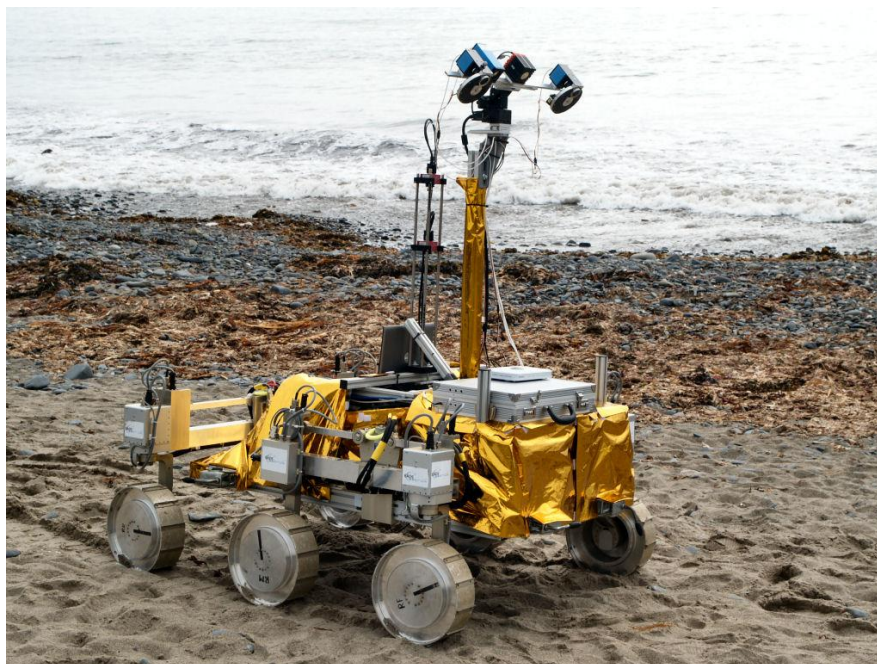
Figure 20: Bridget Rover during the Clarach Bay field trial with mounted optical sensors.
